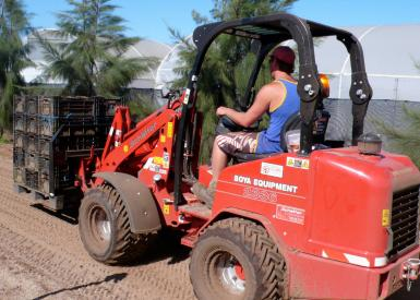
Fuel consumption was extremely economical with the Schaffer 2436 mini digger's fuel consumption during the test period only 2.2L per hour compared to other brands at up to 4.2L per hour.
